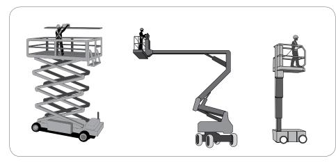
Figure 9: Examples of MEWPS (from left to right): scissor lift, boom lift and vertical personnel platform.
