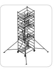
Figure 10: A mobile tower scaffold with access ladder, opening and other features to provide a hazardfree working platform.
