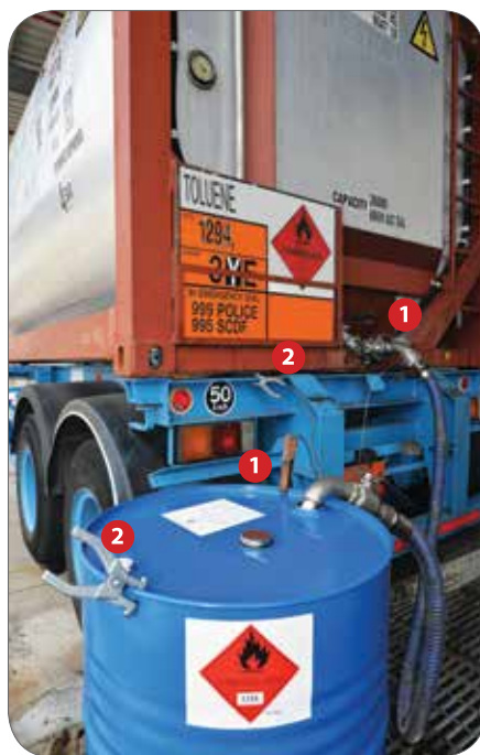
Figure 21: Bonding and grounding of an ISO tank container
