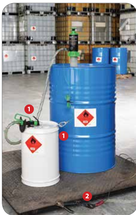
Figure 23: Bonding and grounding necessary for transfer between metal containers
