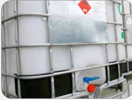
Figure 22: Intermediate Bulk Container (IBC) vs palletised metal drums
