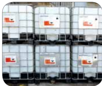
Figure 3: Chemical containers properly stored and labelled.
