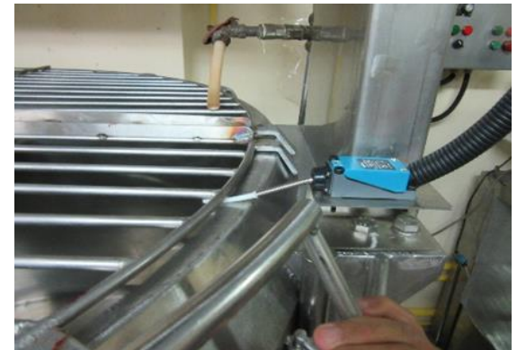
Interlock installed such that mixer will shut off once the cover is lifted
