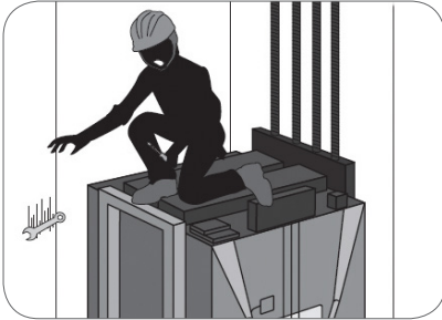
Figure 36: Hand tools falling from lift car top to hoist way
