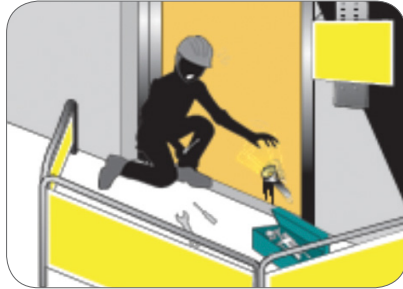
Figure 37: Equipment falling through the landing door to hoist way
