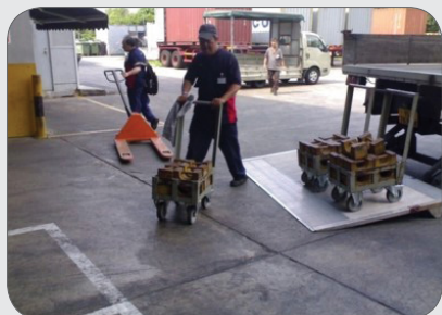
Figure 44: Loading/unloading – test weight (using lorry crane / movable platform / forklift / trolley)
