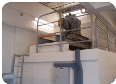
Figure 67: Safety railing to prevent falling from height
