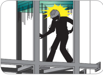
Figure 12: Being trapped between a descending lift car and counterweight inside the hoist way
