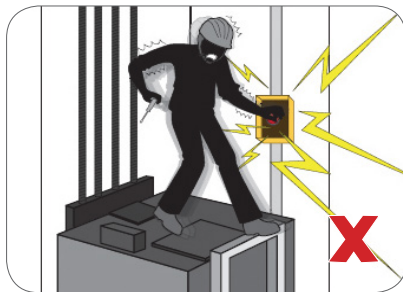
Figure 22: Electrocuted when worker comes into contact with non-finger safe termination blocks
