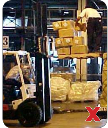
Figure 2: Unauthorised use of forklift to elevate personnel.
