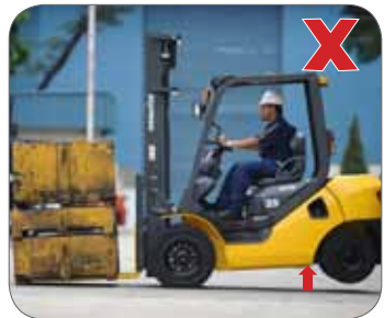
Figure 3: Example of an overloaded forklift.
