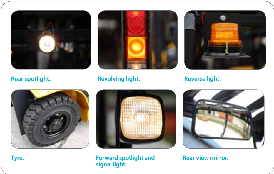
Figure 12: Examples of forklift inspection items.
