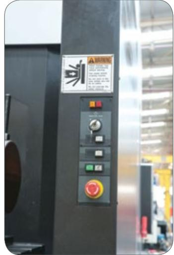
Figure 23: Example of an emergency stop device.
