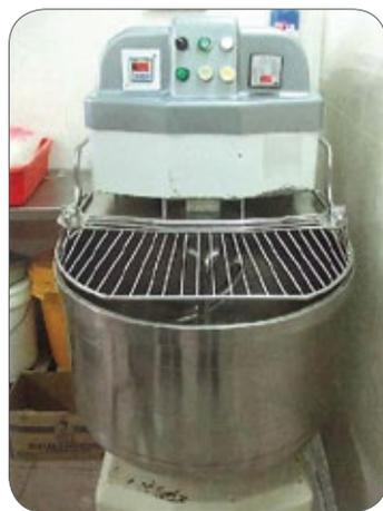
Figure 17: Flour mixer installed with interlocking guard.
