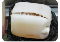
Figure 4: A ruptured waste carboy.
