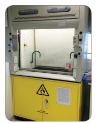
Figure 20: A fume cupboard with a base cabinet specially designed for storage of flammables.
