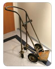
Figure 18: A cylinder cart specially designed for moving gas cylinders.
