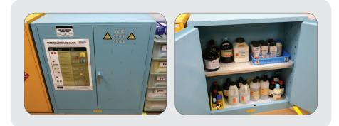
Figure 12: Storage cabinet for corrosive chemicals with cabinet doors closed (left) and open (right).
