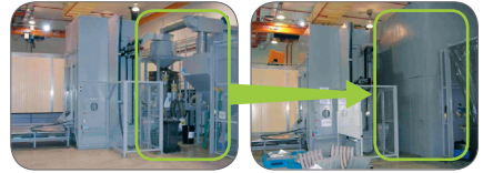
Figure 4: Enclosure of noise generating chamber blast pot.
