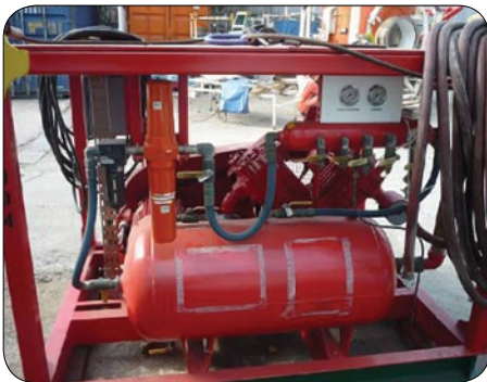
Figure 17: Typical LP air compressor.
