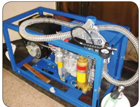
Figure 18: Typical HP air compressor.
