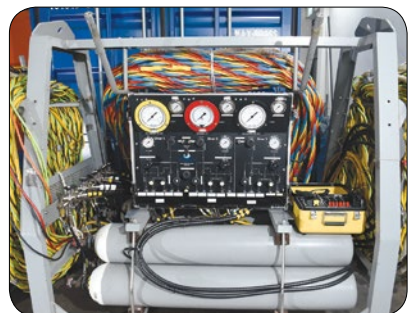
Figure 14: Typical frame-mounted SRP with dive control panel and communication box.
