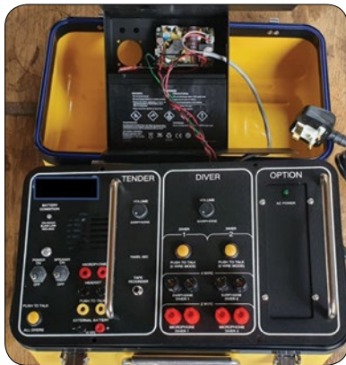
Figure 7: Diver's communications equipment.
