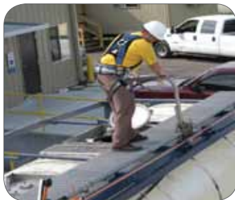
Figure 38: A proprietary TRAM system by Standfast Corp.
