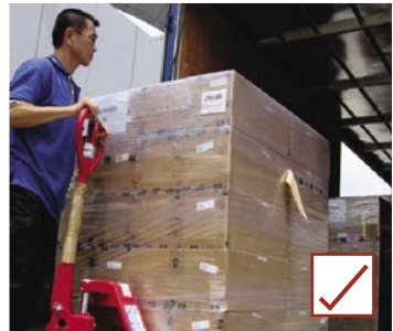
Do not overload or pile loads too high on trolleys
