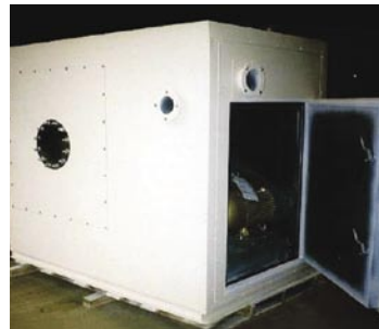
Enclose noisy machinery to reduce the noise in the warehouse
