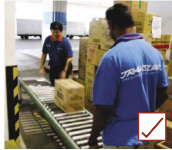
Conveyor belts can help reduce the strain from lifting and carrying
