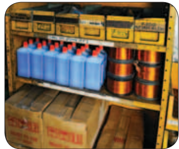
Figure 6: Heavier objects should be stored on the lower shelves for stability and safety.
