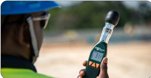
Figure A3: Example of a portable heat index monitor.
