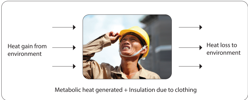
Figure 2: The body gains heat primarily from metabolic heat generation and the environment. Excess heat removal is dependent on the level of insulation due to a worker's clothing and the direction of nett heat exchange with the environment.
