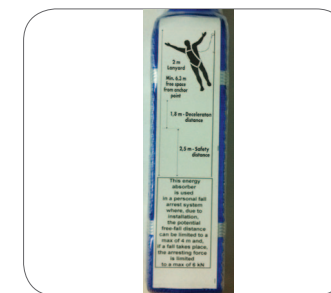
Figure 28: Example of an energy absorber's identity label (opposite side) showing the free fall distance, arresting force and a diagram displaying the safety distance upon activation of the energy absorber.
