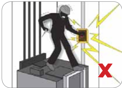
Figure 13: Worker can get electrocuted when he comes into contact with non-finger safe termination blocks.
