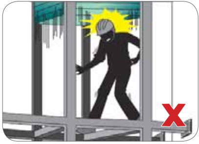
Figure 5: Being trapped between a descending lift car and counterweight inside the hoist way.
