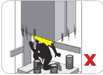
Figure 6: Being trapped between a descending lift car and the bottom of the lift pit.
