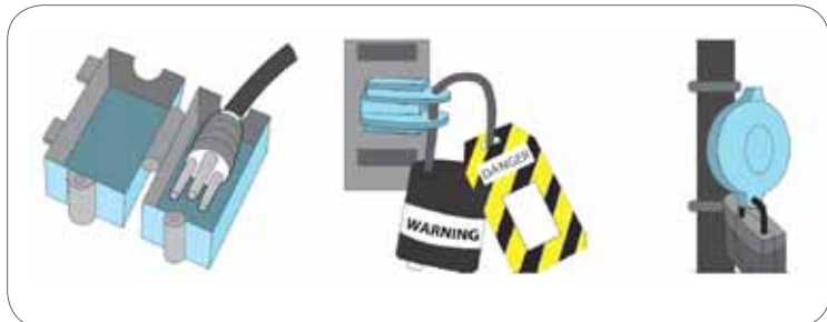
Figure 53: Examples of using lockout and tagout to isolate the source of electrical energy in the machine room.
