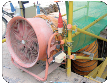
Figure 14: Example of forced ventilation using blower as a mechanical air moving device.
