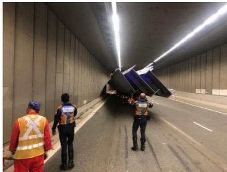
Figure 2: Cargo lopsided due to improper securing of cargo
