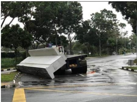
Figure 1: Cargo dislodged while negotiating a bend
