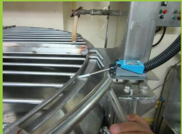
*Figure 2: Mixer with guard cover fitted with interlock switch that cuts off power supply once the cover is open*
