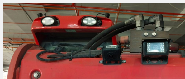
Proximity AI camera mounted on top of the telescopic forklift
