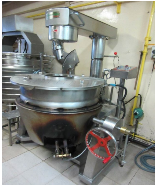
Picture1: Safety interlock installed to ensure cover is closed before operation
