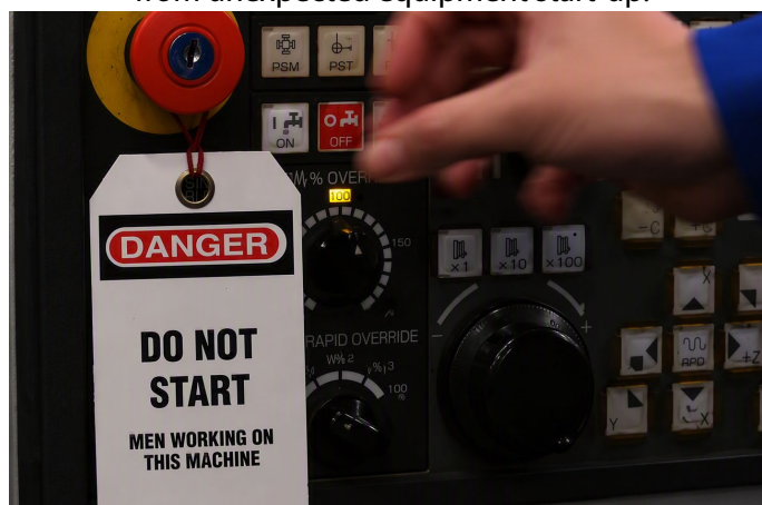
Picture 3: A properly implemented LOTO procedure protects workers from unexpected equipment start-up.
