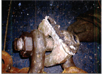
The lifting lug gave way along its welding joint, detaching the elbow pipe.
