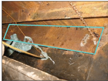
New steel plate to be fitted to the bottom of top side tank.
