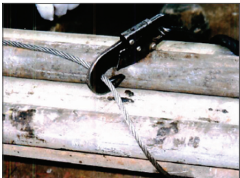
Snap hooks could be left open if not positioned properly.
