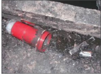
Shattered battery operated torch found in the water ballast tank.
