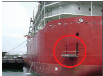
Hanging scaffold that the deceased and his co-worker were dismantling, on the bow of a vessel.
