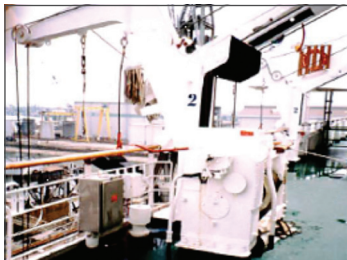
Winch system which was used to lower the lifeboat.
