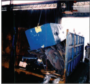
Side view of the overhead crane, chain sling, scrap box and dumping container.
