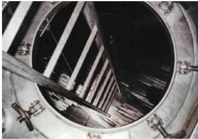
Figure 1: Close-up of the manhole opening at the top of the ISO tank.
