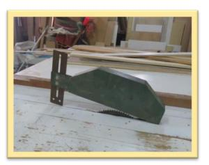
Pic 3: Table saw guard was available but was removed prior to the accident
