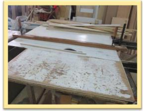
Pic 2: Guard was not installed during the day of accident
