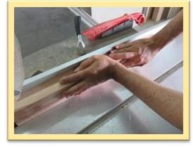
Pic 4: Table saw guard was available but was removed prior to the accident.
