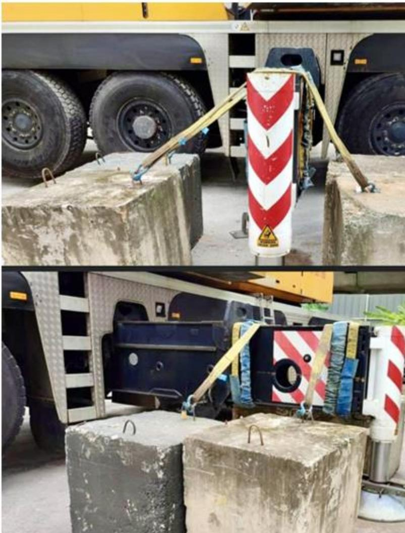
Photos show concrete blocks and slings being used to hold down an extended crane outrigger
