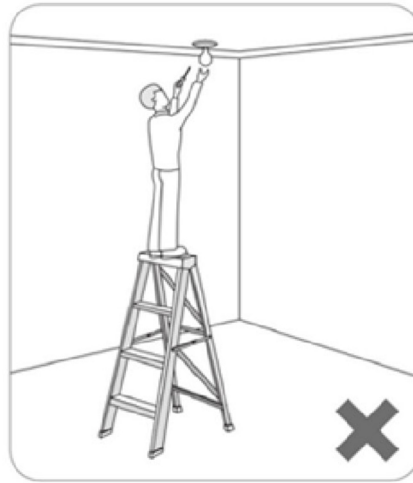
Figure 7: There is a high risk of falling when one stands on the top rung of an A-frame ladder.
