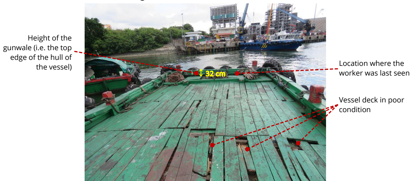
Figure 1: Scene of the accident.
