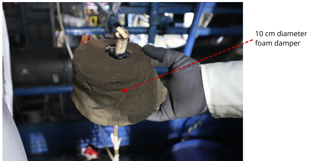
Figure 4: The foam damper used at the bottom end of the 10 cm pipe.
