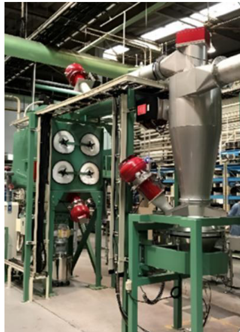
A dust collector with an explosion-suppression system.
