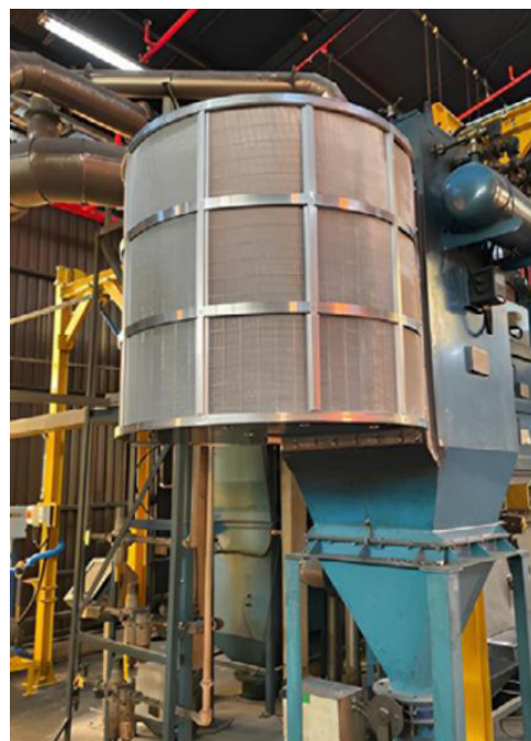
Flame-free explosion vent. Check that pressure relief from the vents are directed away from people and critical equipment.
