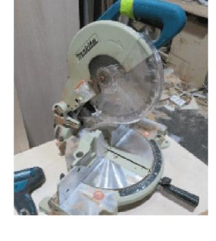
A self-adjustable blade guard on a circular saw which retracts when the sawblade is moved downwards for cutting works and automatically springs back to cover the blade once the cutting is done.
