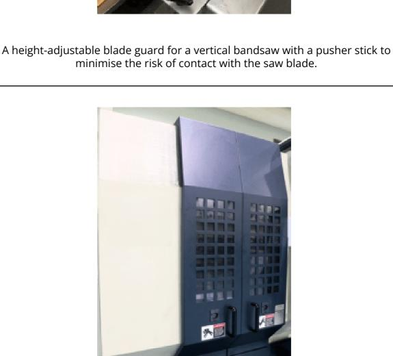
A machine where the movement of its internal parts will automatically stop once its doors are opened.
