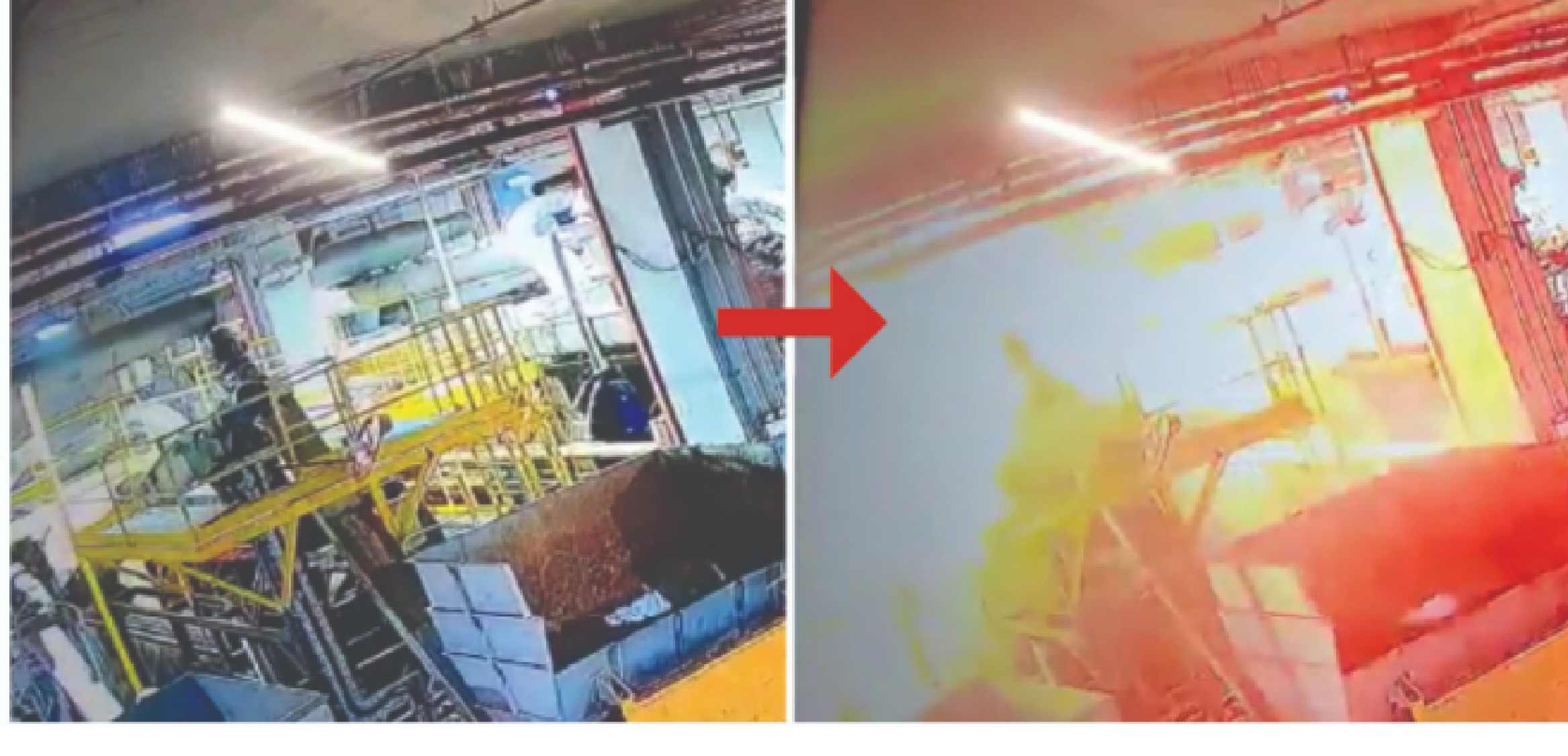
Figure 1: Dryer machine used to dry spent grains. CCTV footage confirmed a flash fire had occurred.
