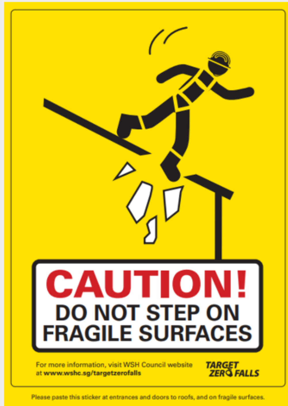
Figure 2: Example of fragile surface warning sign.
