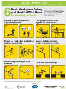
6 Basic Workplace Safety and Health Rules for Working on Roofs
