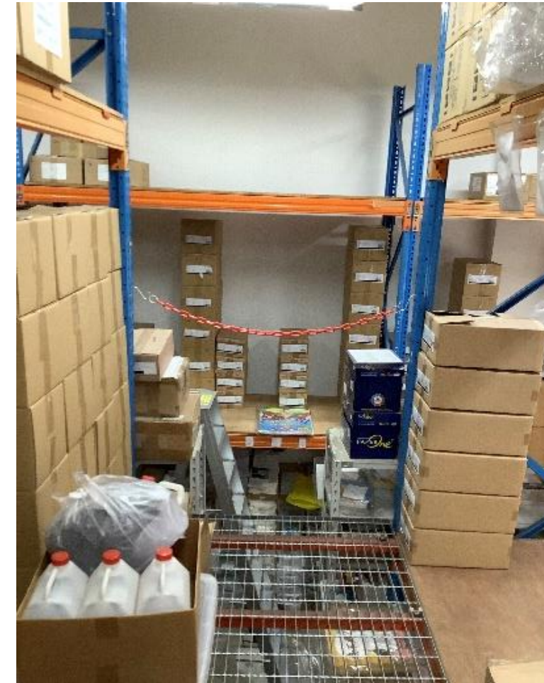
Ineffective barricades and unsafe means of access and egress
