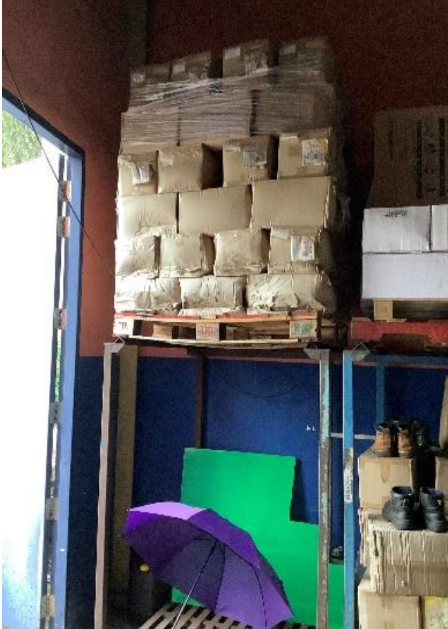
No SWL and inadequate support
