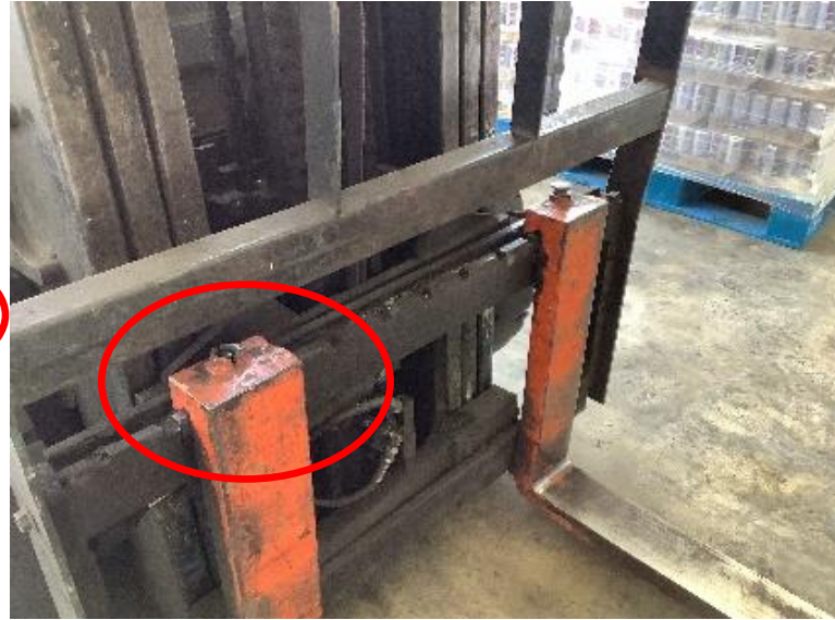
Damaged locking pin
