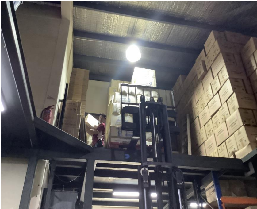
No barricades and travel restraint system
