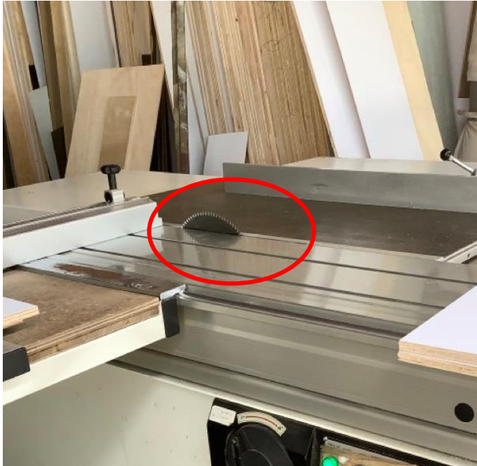
Moving/rotating parts of machine not guarded
