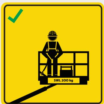
Anchor the harness to the designated anchor point when working on MEWPs.
