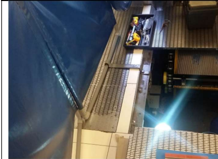
Figure 25 : Tools not being secured
