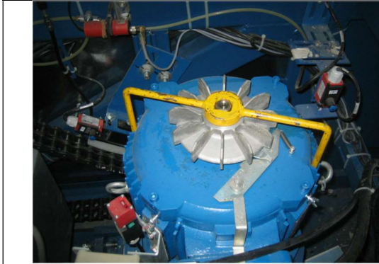
Figure 39 : Brake release tool to be applied
