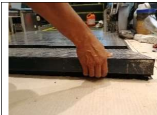
Figure 4: Fingers pinched by floor plates
