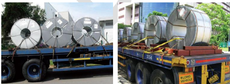
Figure 46: Sheet metal rolls chocked with dunnage (left) loaded within metal brackets (right).
