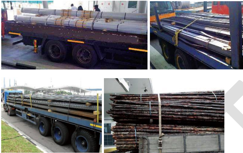
Figure 38: Various long cargo bundled and lashed.
