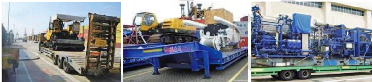
Figure 53: Transporting heavy machines on low bed trailers.
