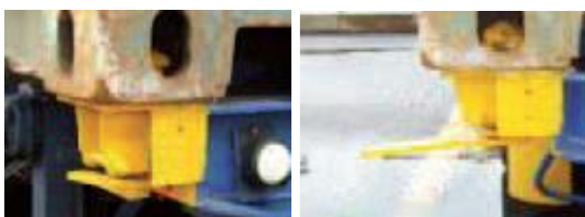
Figure 29: Twistlocks in locked and unlocked positions.
