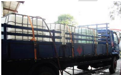
Figure 44: Intermediate bulk containers secured with lashing.
