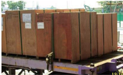
Figure 42: Lashing on boxes.
