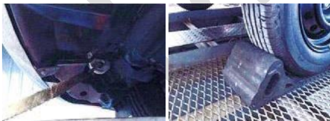
Figure 52: Anchorage point under a car (left) and wheel chock (right).
