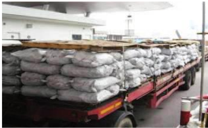
Figure 36: Sacks loaded in alternating directions.
