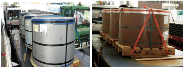
Figure 47: Coiled sheet metal loaded on pallets and lashed.
