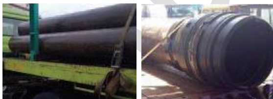
Figure 50: Steel pipes loaded against stanchion and lashed to loading platform.
