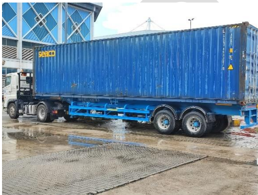
Figure 24: Trailer fitted with ISO container.
