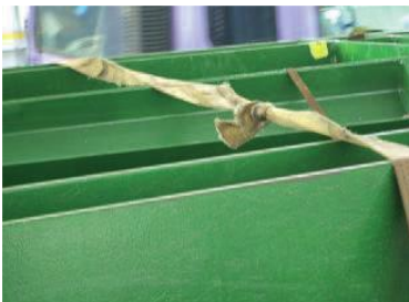
Figure 22: Bad practice of tying two lashing belts.
