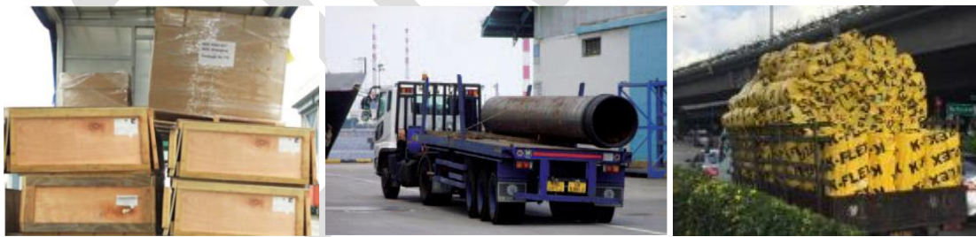
Figure 7: Examples of poor cargo arrangement. (From left to right: unstable stacking, unbalanced weight distribution, cargo stacked higher than headboard.)
