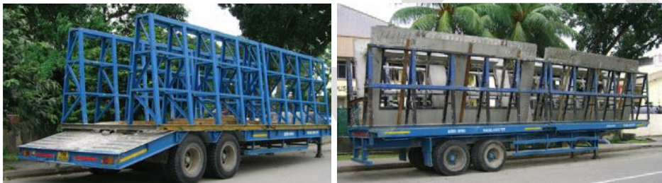
Figure 55: Trailers mounted with steel frames for transporting precast concrete.
