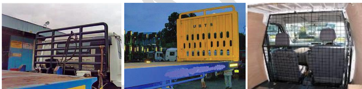
Figure 11: Cabin guards (left, middle) and front bulkhead (right).
