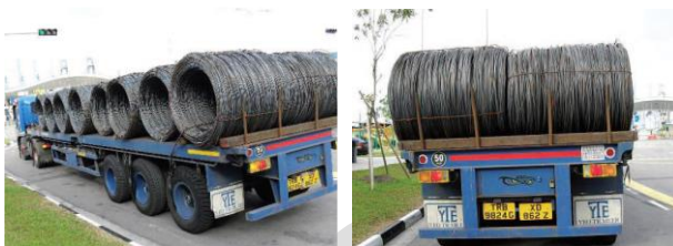
Figure 45: Wire coils lashed and blocked with a metal bracket at the rear.
