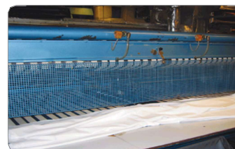
Figure 8: Example of a machine guard in the laundry.
