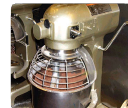
Figure 9: Example of a machine guard.
