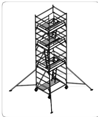
Figure 22: A mobile scaffold with access ladder, opening and other features to provide a hazard-free working platform.
