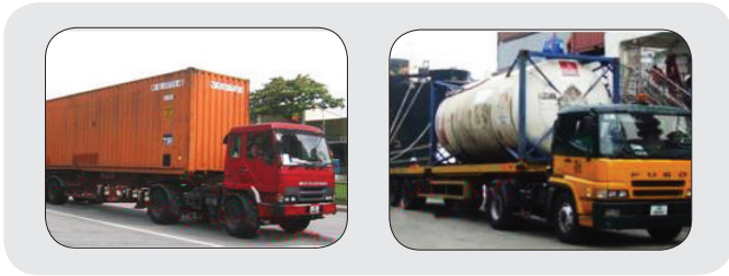
Figure 54: ISO container (left) and ISO tank (right).
