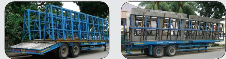
Figure 53: Trailers mounted with steel frames for transporting precast concrete.
