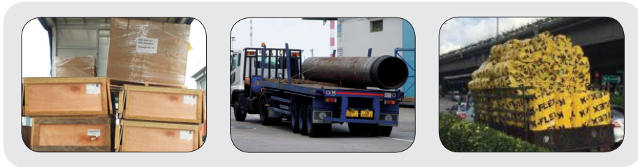
Figure 6: Examples of poor cargo arrangement (from left to right): unstable stacking, unbalanced weight distribution, cargo stacked higher than headboard.
