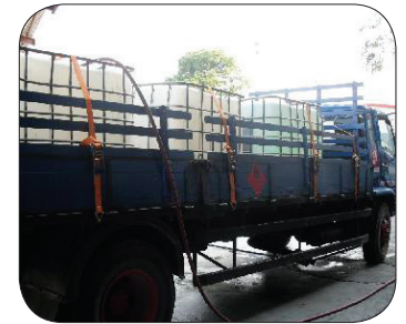
Figure 41: Intermediate bulk containers secured with lashing.
