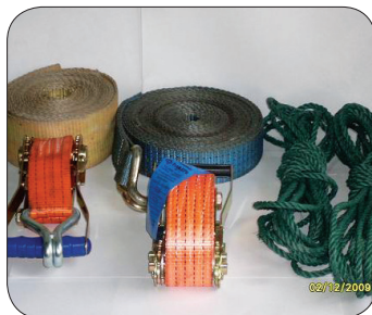
Figure 18: Lashing belts (webbing) and polyester rope.
