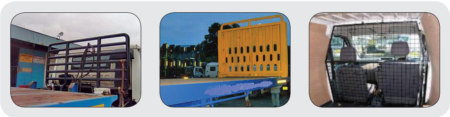
Figure 8: Cabin guards (left, middle) and front bulkhead (right).
