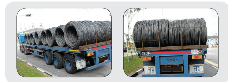
Figure 42: Coils of wire lashed and blocked with a metal bracket at the rear.
