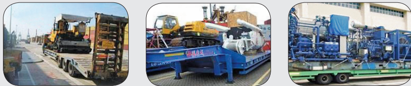
Figure 51: Transporting heavy machines on low bed trailers.
