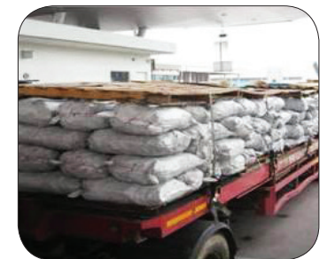
Figure 33: Sacks loaded in alternating directions.
