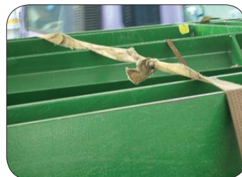
Figure 19: Bad practice of tying two lashing belts.
