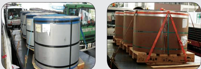
Figure 44: Coils sheet metal loaded on pallets and lashed.
