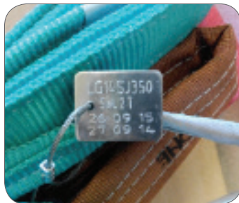
Figure 17: Webbing with tag displaying safe working load.
