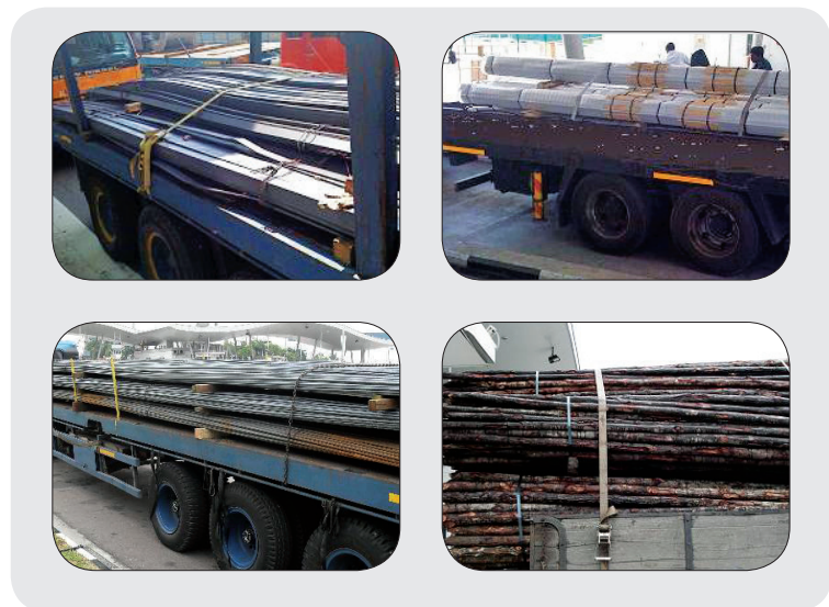
Figure 35: Various long cargo bundled and lashed.
