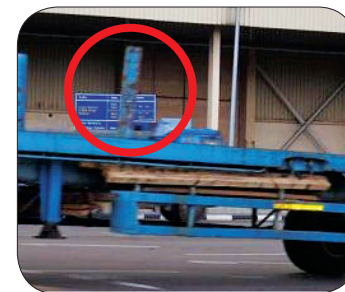
Figure 12: Stanchion bars on a trailer bed.
