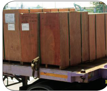
Figure 39: Lashing on boxes.
