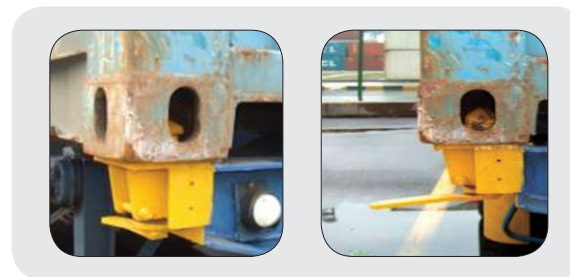
Figure 26: Twistlocks in locked and unlocked positions.
