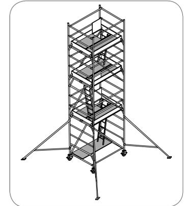
Figure 10: A mobile tower scaffold with access ladder, opening and other features to provide a hazard-free working platform.
