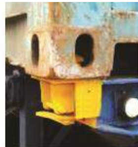
Twist lock in locked position
