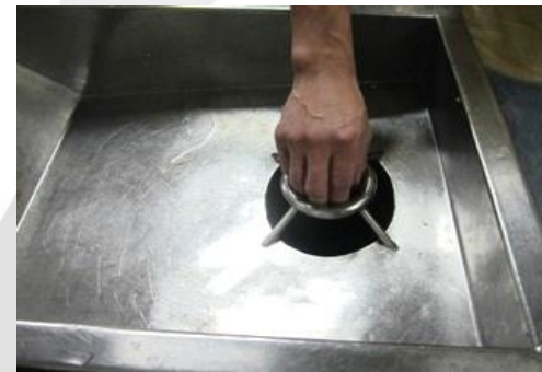
Figure 6b. Guarding installed to protect hands and fingers from contact with the rotating worm
