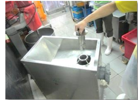
Figure 6c. Push stick specially designed to go through the guarding and towards the rotating worm
