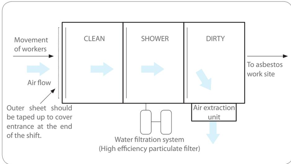
Figure 14: Illustration of a decontamination facility equipped with a high efficiency particulate filter and air extraction unit.
