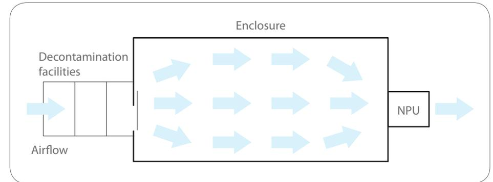
Figure 11: Illustration of an enclosure with an NPU.
