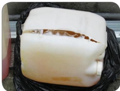
Figure 4: **A ruptured waste carboy.**
