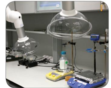
Figure 19: A flexible arm capture hood can be positioned close to the contaminant source.
