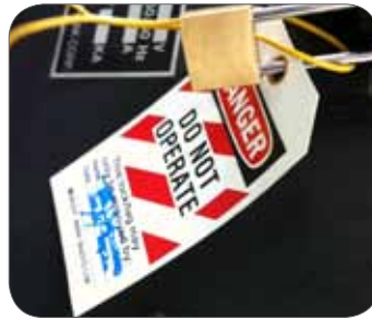
Figure 8: Machine locked-out and tagged-out for maintenance.
