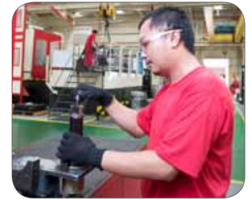
Figure 6: Example of PPE being used: Worker wearing gloves when working with hand tools.
