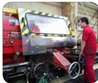
Figure 5: Example of an engineering control: Machine guarding installed on moving part of machine.
