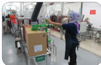
Figure 1: Using a vacuum lifter to lift heavy objects.
