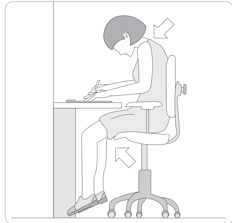
Figure 8: Awkward sitting posture at the office workstation can potentially lead to MSDs in the areas indicated by the arrow.
