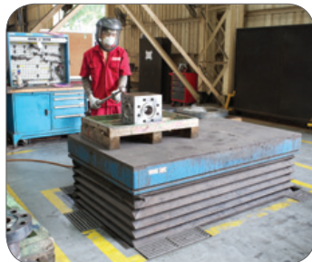
Figure 9: Use an adjustable table to adjust the height of the work platform.
