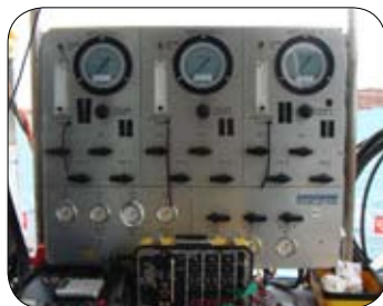
Photo 7 : Typical divers communications equipment.
