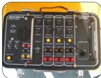
Photo 7 : Typical divers communications equipment.
