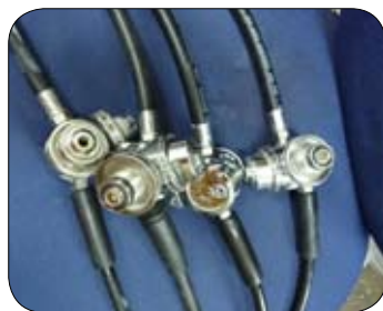
Photo 15 : Divers bail out bottle first stage regulators.
