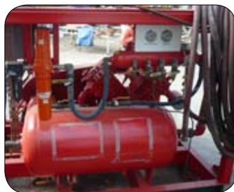
Photo 18: Typical LP air compressor.
