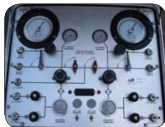
Photo 5 : Typical portable air supply panel.
