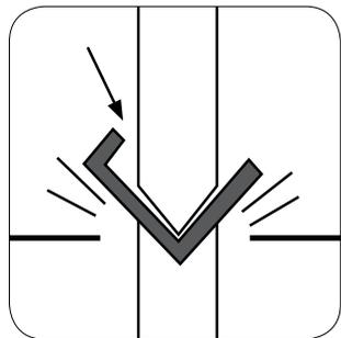
Figure 2: Metal sheet bends and creates “caught in between” hazards
