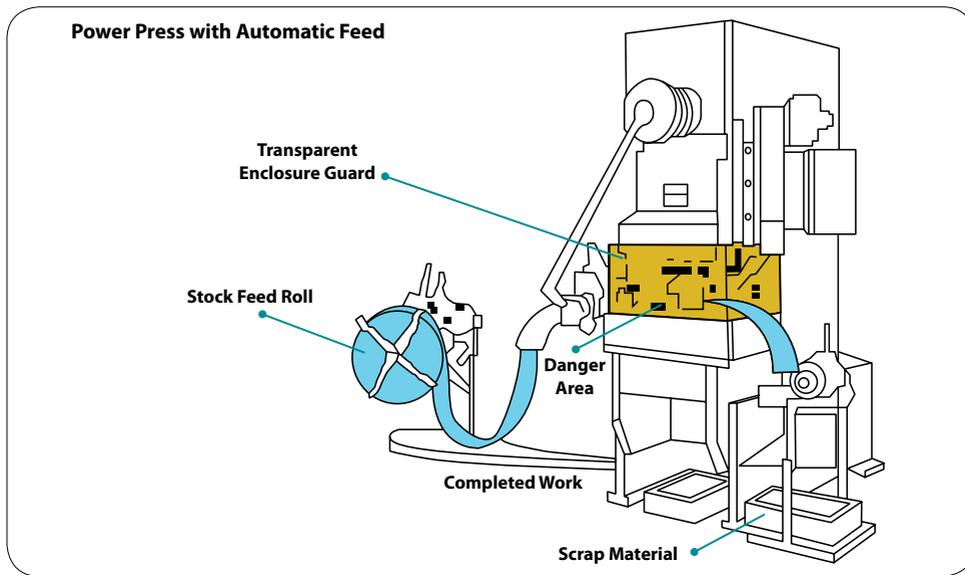
Figure 6: Entanglement can happen during a stock feed
