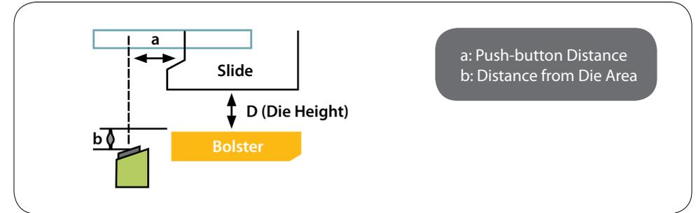
Figure 16: Distance of two-hand control away from die area.
