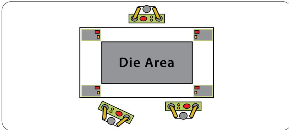
Figure 18: Two-hand control buttons
