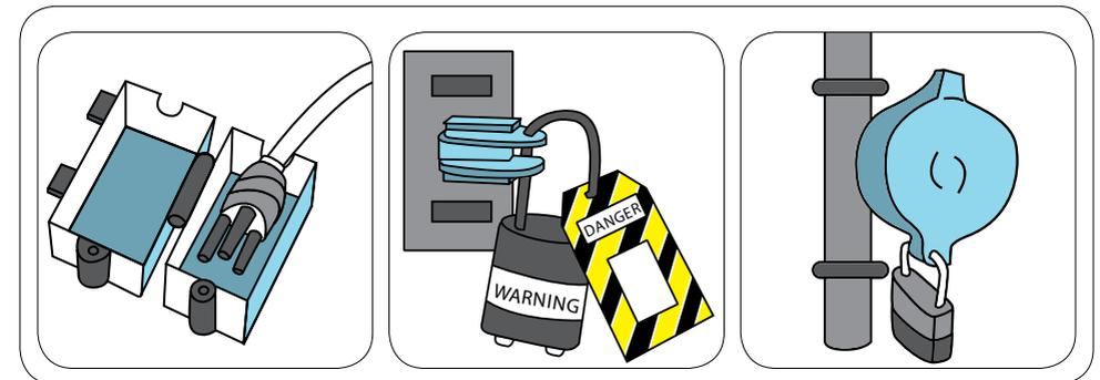
Figure 13: A variety of lockout devices
