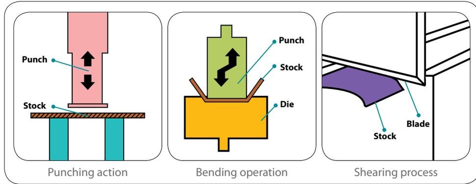
Figure 1: Power press operation
