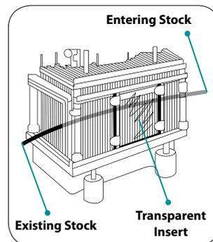
Figure 7: Fixed barrier guard
