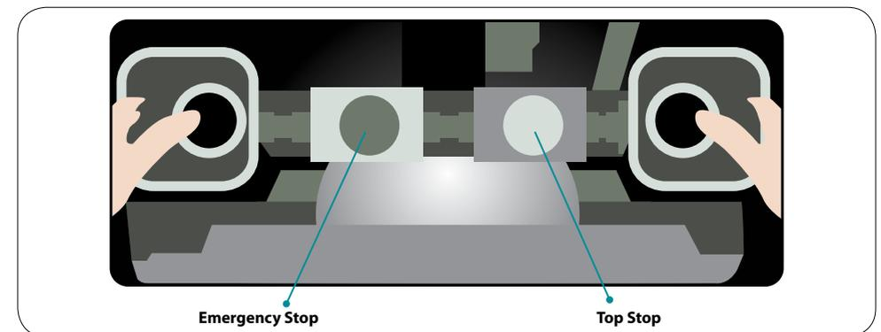
Figure 11: Two-hand control device
