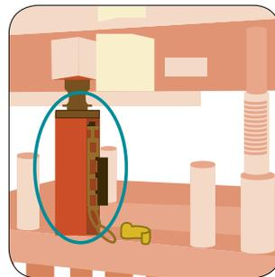
Figure 4: The use of a safety block
