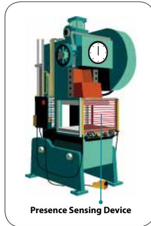
Figure 9: Presence-sensing safety device on power press
