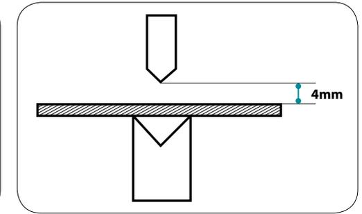
Figure 21: Gap opening between work piece and tool/die
