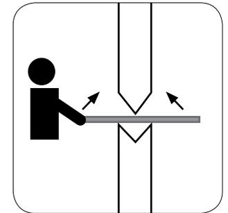
Figure 5: Metal piece “slapping” operator
