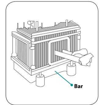
Figure 8: Power press with adjustable barrier guard
