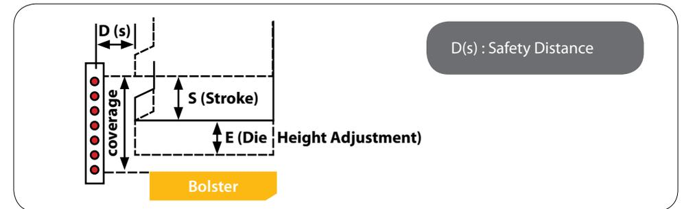
Figure 17: Distance of safety light curtain to die area
