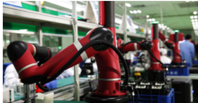
Fig 2: Example of collaborative robots that can operate without causing injury to workers in the vicinity. (Photo courtesy of Rethink Robotics Inc.)
