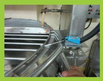
Figure 2: Mixer with guard cover fitted with interlock switch that cuts off power supply once the cover is open
